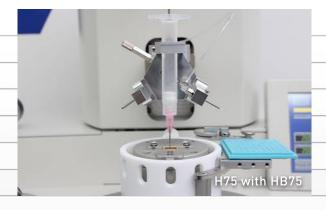
The H75 dispenser kit includes a digital dispenser controller, syringe, holder, tubes and needle tips.
