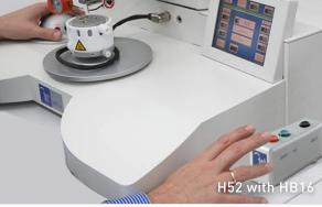
The TPT dynamic search box offers 3 features: manual approaching the substrate surface with small steps for better aiming, manual raising or lowering the search height in 30µm steps to bond the second bond on a different bond height and connecting single wedge bonds to a series of stitch bonds.
