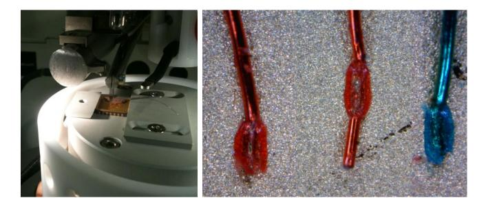
wedge in transducer with wire piece
