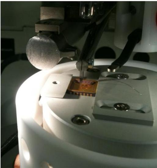
wedge in transducer with wire piece
